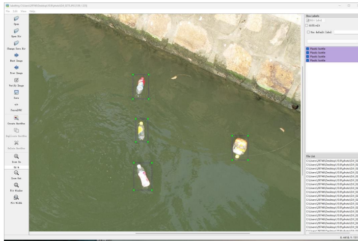
Figure 3: Image labeling steps for plastic bottles using LabelImg
