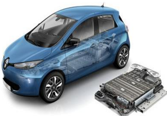
Fig.4: Lithium-nickel-manganese-cobalt battery systems of the Renault ZOE with a range of 403 km
