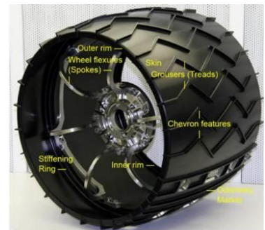
Figure 1. Curiosity's wheel made from a single piece of machined aluminum alloy AA7075-T7351. The main rim is 1.9 cm thick (0.75-inches).
