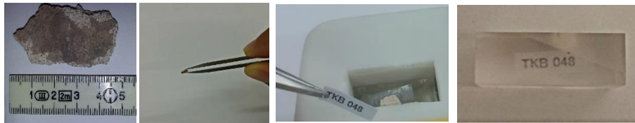
Fig. 2 Showing The preparation of the cross-section steps for microscopic observations
