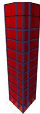
Fig.7 Model of G+10 frame with infills
