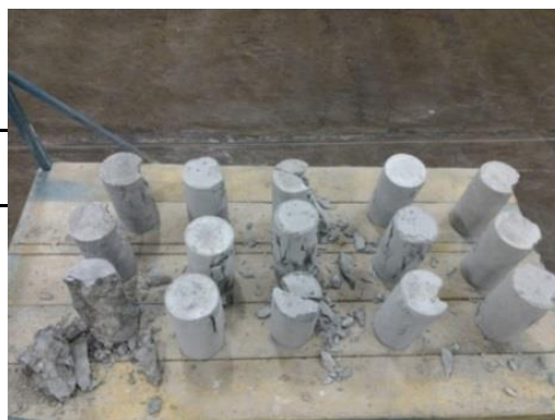
Fig. 1. Test specimens of concrete tested in compression
