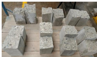
Fig. 5. Test specimens of concrete tested in compression
