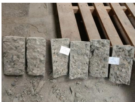
Fig. 3. Specimens of concrete tested to traction
