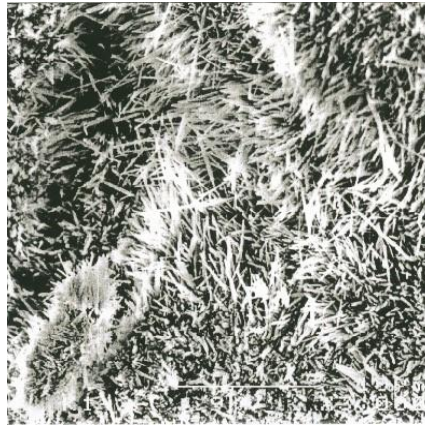
Figure 2. Scanning electron microscopy Micrograph of kaolinite sample .
