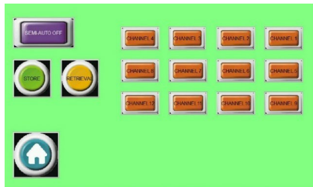
Fig. 8. Semi-Auto Mode, users can select the desired slot and choose to store or retrieve pallet.
