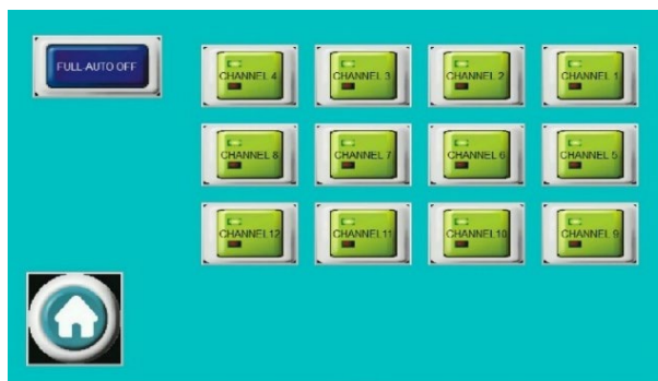
Fig. 9. Full Auto Mode, users only selected the desired slot and the system will operate every step.
