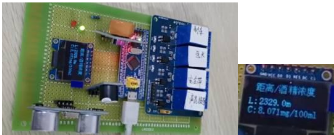
Figure 3 oled display L: distance from the front obstacle C: air alcohol concentration
