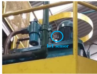
Fig. 5. Motor 3,7kW/ 4 poles/ 380V/ 60Hz/ 1730rpm/ Frame IEC100L/ \eta=83,5\% / Application: pump.
