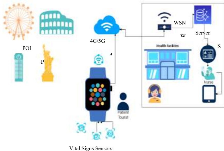
Fig 2 - Health Tourist Monitor System Architecture
