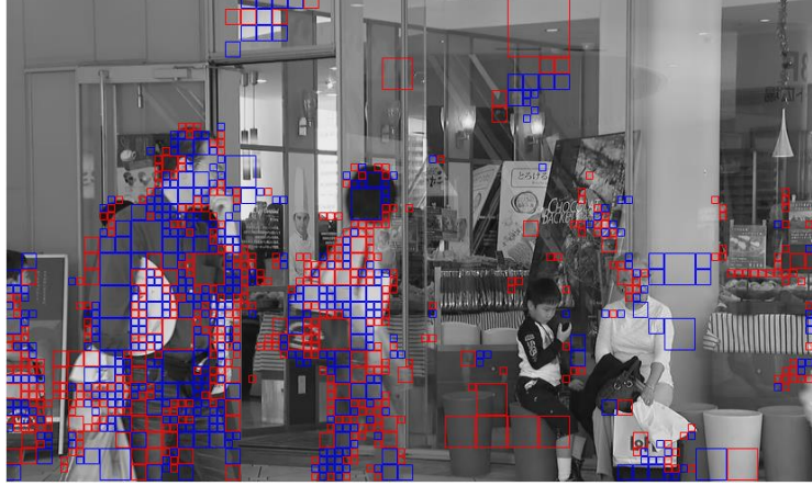
Fig. 4. Visualization iCNN/DCTIF interpolation selection on POC7 of sequence BQMall. Blue, red blocks represent for CU that choose DCTIF, iCNN, respectively. The other parts include intra-coding CUs and CUs have integer MVs.
