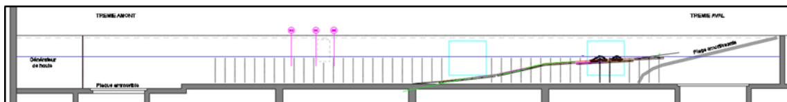
Figure 3: Section of the wave flume. The piston-type wavemaker at left. The gauges are represented in fuchsia color, the two rectangles of blue color represent the two windows of the canal, the model is visible at the level of the right window, the sloping beach on the far right is not utilized, the gray vertical lines represent the fixing rails of the adjustable elements, the concrete structure of the wave channel is illustrated by the broad gray lines.
