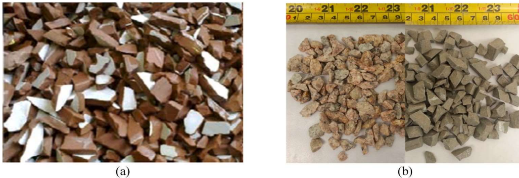
Fig. 2. (A) Ceramic Aggregate's flaky shape; (B) Ceramic Aggregate's (right) angular and uneven shape in comparison to natural Aggregate (left)
