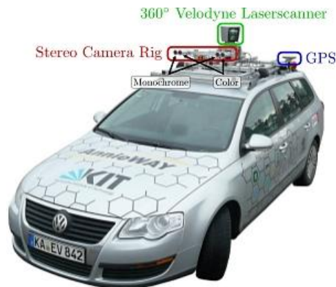
Figure 3.4: Autonomous Driving Platform for KITTI
